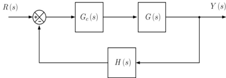
where the plant  $G(s) = \frac{G_o}{1 + \frac{s}{Q\omega_o} + (\frac{s}{\omega_o})^2}$ ,  $G_o = 50$ ,  $Q = 1.66$ ,  $\omega_o = 2\pi(1000)$  and  $H(s) = \frac{1}{2}$ .
